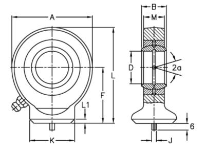
$\begin{array}{lll} A & = 92 \\ a \ (degrees) & = 7 \\ B & = 28 \\ D & = 40 \\ Dynamic \ load \ C \ (kN) = 100 \\ F & = 69 \\ J & = 4 \\ K & = 52 \\ \end{array}$
